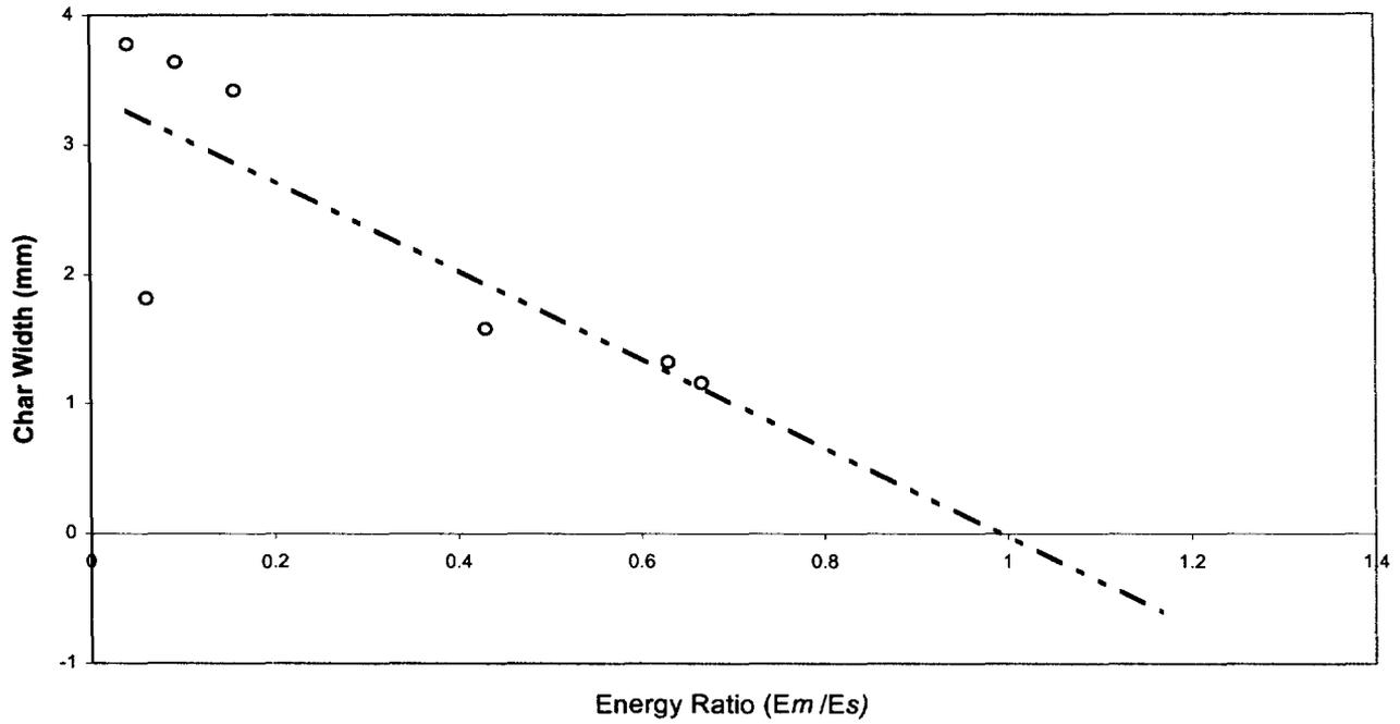
*Fig. 3. Laser power on 60W. Velocities vary. Length of cut, Kerf width and depth are measured to determine energy required to cut. Energy ratio is efficiency of laser interacting with substrate. No shielding gas used on bottom surface.*
