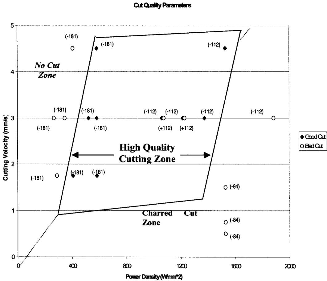
Fig. 7. Quality cutting zone chart. Numerical data in parenthesis refer to spot radius in microns and the plus and minus signs refer to the focal plane (beam waist) location as listed in Table 2. Dark circles are good cuts. Top and bottom boundaries on Quality cutting zone are estimated.
