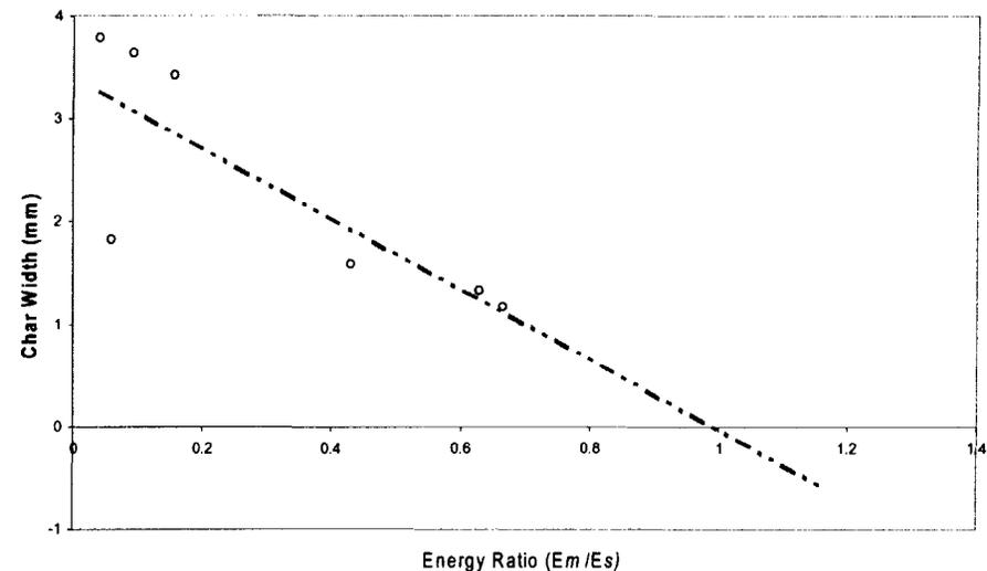
*Laser power on 60W. Velocities vary. Length of cut, Kerf width and depth are measured to determine energy required to cut. Energy ratio is efficiency of laser interacting with substrate. No shielding gas used on bottom surface.*
