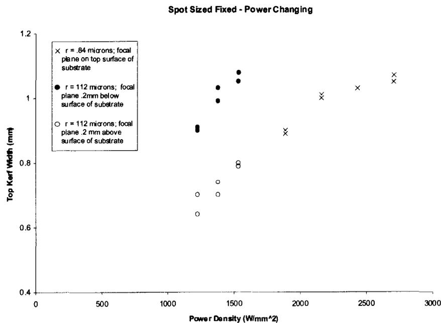
*Kerf width for 3 different focal positions. Velocity (3 mm/s) and gas (100Kpa) are constant. Note different kerf width for same power density because of the different focal plane orientation (above or below surface).*
