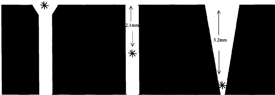
*Fig. 4. Cut profile with focal plane at 3 different locations. Left to right; top surface of material, center of material (2.1mm below surface), near bottom surface of material (3.2mm below surface).*
