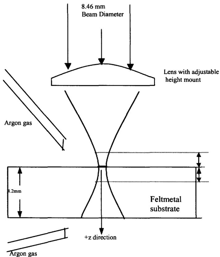
*Fig. 1. Diagram of experimental setup. Spot size on surface of feltmetal changed by raising and lowering asphere lens.*
