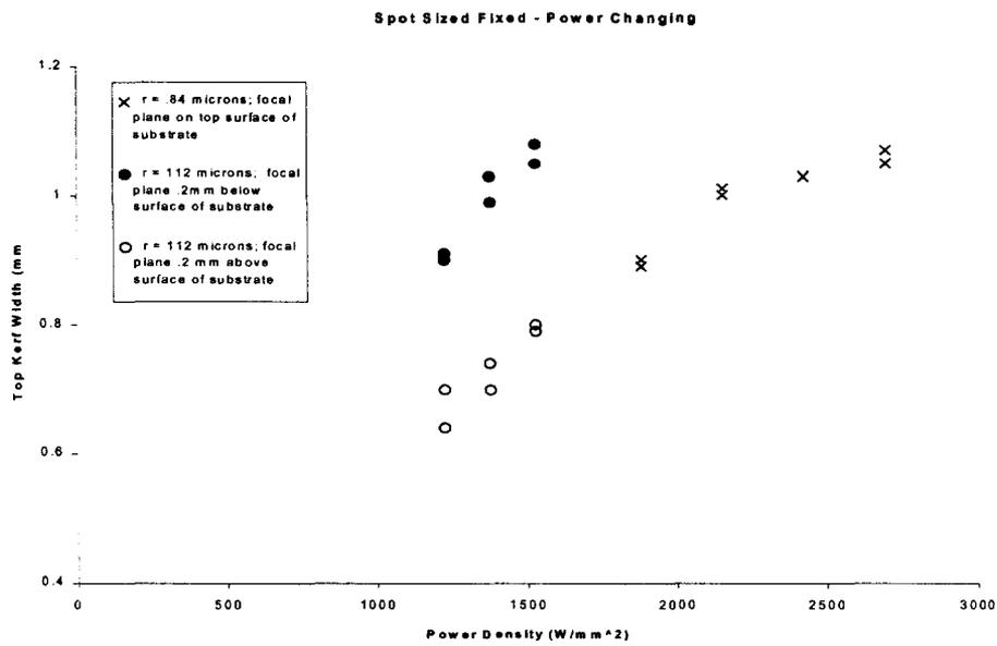
*Fig. 6. Kerf width for 3 different focal positions. Velocity (3 mm/s) and gas (100Kpa) are constant. Note different kerf width for same power density because of the different focal plane orientation (above or below surface).*
