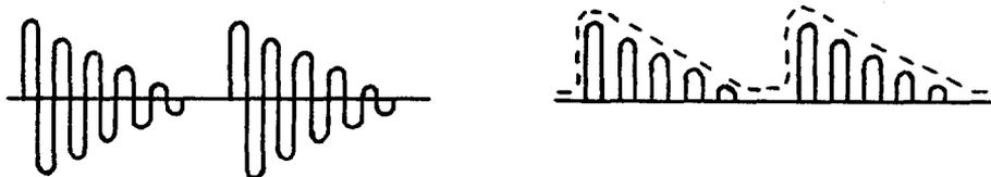
Figure 4: Oscillation and Rectified Oscillation
