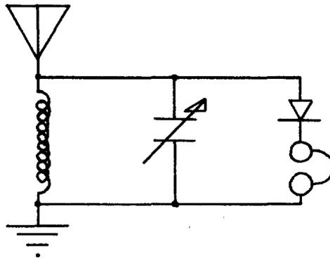
Figure 3: Crystal Radio In Schematic
