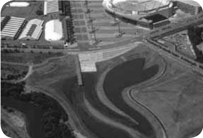
14. SYDNEY OLYMPIC PARK Sculptural wetland feature that filters surface water before releasing it into the natural watershed. (Photo by Hargreaves Associates)
