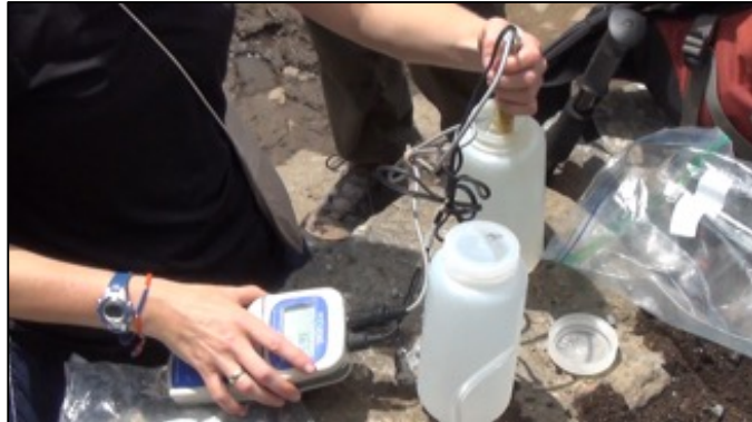
Figure 5a- Sample taken in Whirlpak bag in front of water source for drinking and washing clothes. (Photo credit: Emily Hayes) Figure 5b- Analyzing water samples in the field for physical parameters using a FisherSci Ap85 portable meter. (Photo credit: Kirsten Nicholson)
