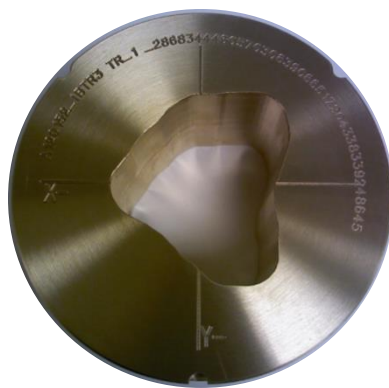
Figure 1.4: Aperture. The aperture is a device that will be inserted into the treatment field on the snout. The aperture shapes the lateral edges of the treatment field.
